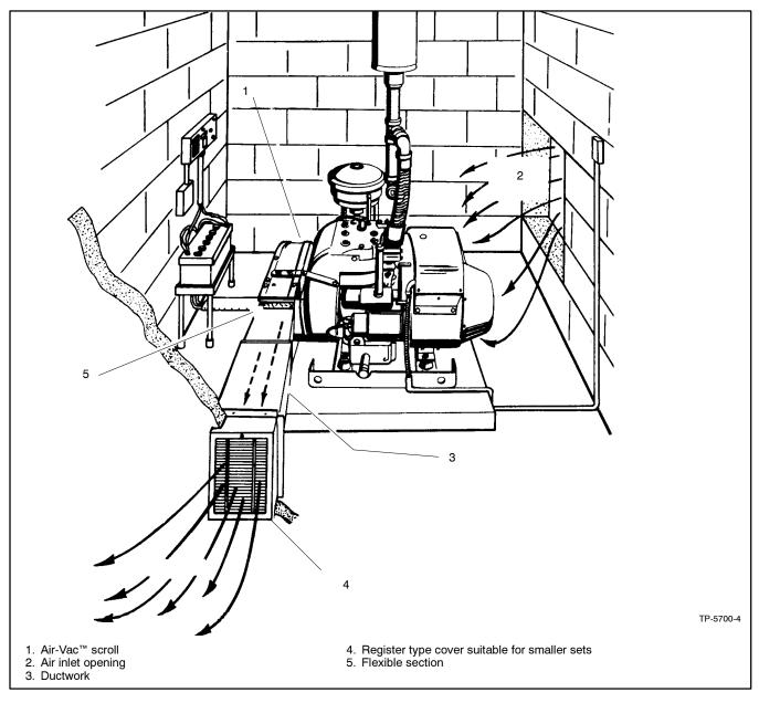
Figure 4-6 Air-Vac™ Cooling System
